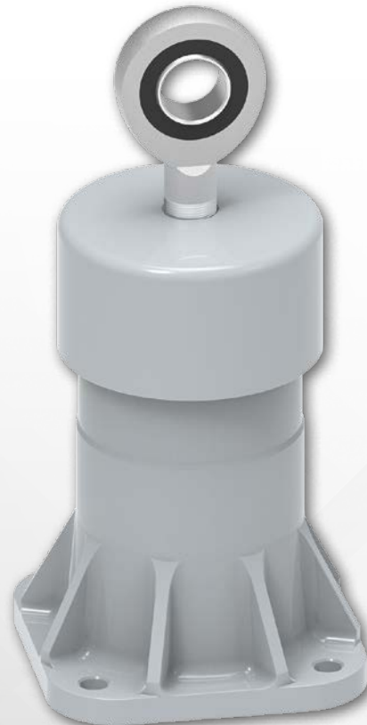
Fig. 4: Push-Pull Units for protection against earthquake-induced damage by decoupling surge arresters from the base foundation
