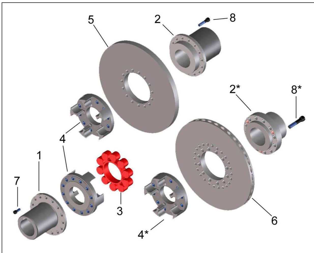
Fig. 1 Construction RINGFEDER® TNS SDDL-5-BS
