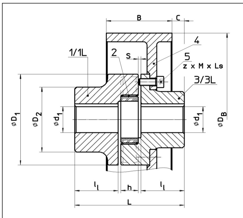
Fig. 2 Construction RINGFEDER® TNS S-BT
