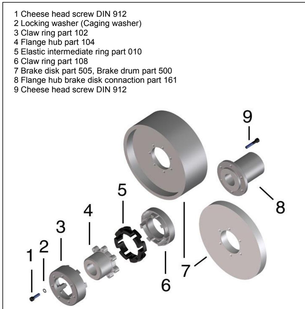
Fig. 1 Construction RINGFEDER® TNM GHBS
