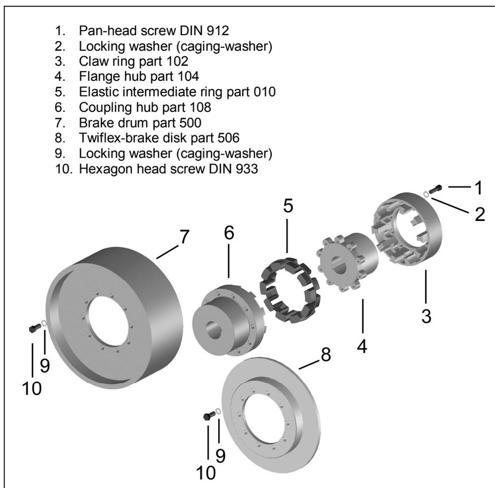
Fig. 1 Construction RINGFEDER® TNM GBT, TNM GTW
