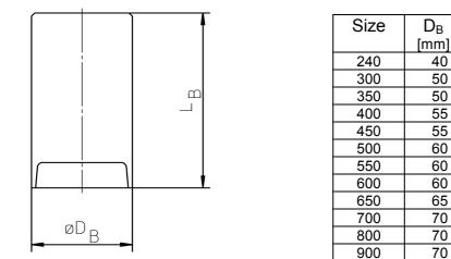
In case of particularly high balance requirements, the elastic buffers are weight balanced per set.
