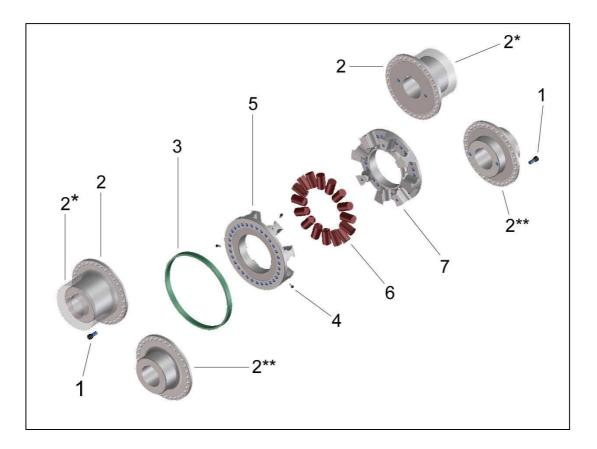
Fig. 1 Construction RINGFEDER® TNB BHDD, TNB BHDDV, TNB BHDDVV
