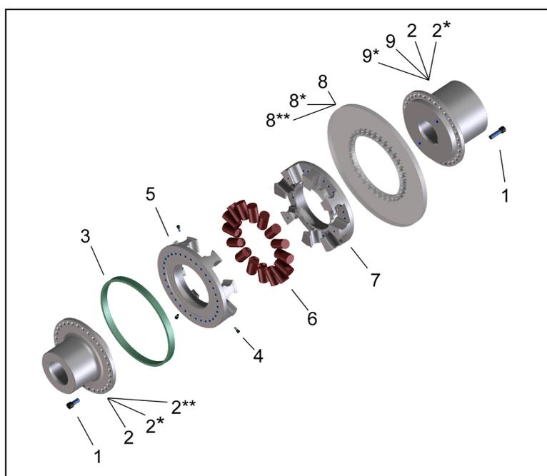
Fig. 1 Construction RINGFEDER® TNB BHD-BS
