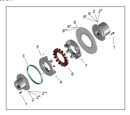
Fig. 1 Construction RINGFEDER® TNB BHD-BS
